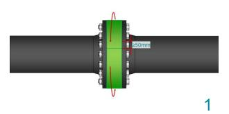
Ensure a proper surface preparation prior to the application of Wrappingband. Apply a straight wrap of Wrappingband over the flange.
