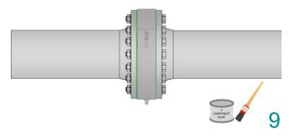
Paint the bolts and pipelines with a thick layer of an appropriate paint according client specification.
