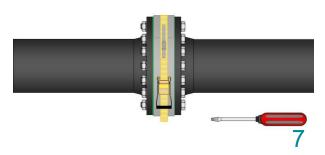
Tighten the Flangebelt with a ratchet strap. Tighten the clamp frequently during the strapping process.
