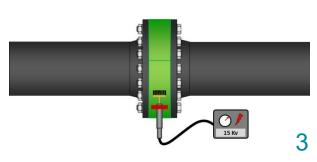
A holiday test using a high voltage tester must be carried out on the green Stopaq Wrappingband prior to the application of any Outerwrap. The test must be carried out at a minimum of 15kV.
