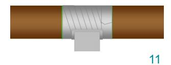
Outerglass Shield XT can be coated with a topcoat at above ground pipe supports.
