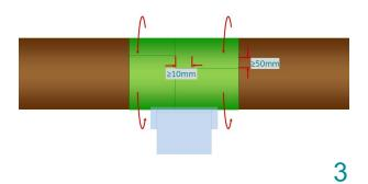
Apply Wrappingband with straight wraps. Side-byside overlap minimum 10mm. Number of wraps depending on the size of the pipe support.
