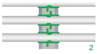
Apply without air enclosures and firmly press the materials in all corners, underneath and around the pipe into the pores of the substrates.
