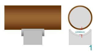
Ensure a proper surface preparation prior to the application of Wrappingband. Pre cut strips of Wrappingband corresponding to the pipeline circumference + approx. 100mm on larger diameter pipelines and approx. 50mm on smaller diameter pipelines.
