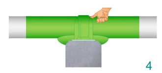
Apply without tension and avoid air enclosures. Check the adhesion on a regular base.
