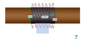
Start application of Outerwrap with 2 straight circumferential wraps and continue by means of spiral wrap with a minimum overlap of 50%. Finish with 2 straight circumferential wraps.
