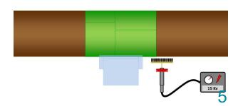
A holiday test using a high voltage tester must be carried out on the green Stopaq Wrappingband prior to the application of any Outerwrap. The test must be carried out at a minimum of 15kV.
