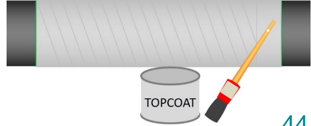
Outerglass Shield XT has to be painted with an UV resistant topcoat for above ground applications.
