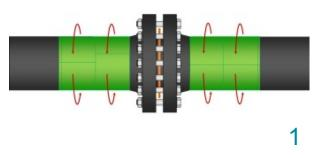
Ensure a proper surface preparation prior to the application of Wrappingband. Apply Wrappingband on the pipe with straight or spiral wraps on each pipe section connected to the flange. Start touching the flanges. Width according to client specification.
