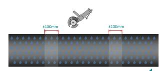
Clean 2 circumferential bare metal rings of 100mm wide at both extremities of the area to be coated with Wrappingband CL. Rinse the pipe with clean water. Ensure a proper surface preparation, minimum St2-St3, prior to the application of Wrappingband CL.
