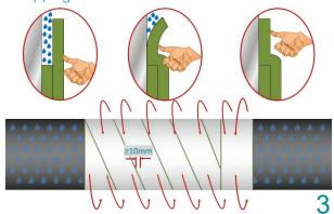
Apply Wrappingband CL with a minimum overlap of 10mm. Avoid air and water inclusion by pressing the material firmly onto the surface and on the seam of the overlap. Do not remove the white backing foil, remove the transparent release foil only.
