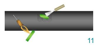
Preheat some Paste and mould it into the damaged area without air inclusions. Avoid smearing Paste beyond the damaged area.
