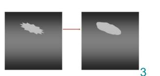
Remove loose coating and bevel all sharp edges of the coating damage.
