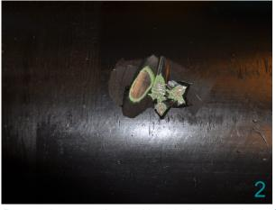
Remove loose coating and bevel all sharp edges of the coating damage.
