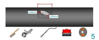
Roughen the surface of the plant coating around the damaged spot with an abrasive pad or sand paper. Remove all contaminations.
