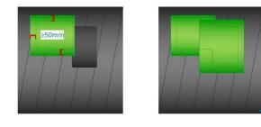
Depending on the size and depth of the damage, Paste might be necessary to fill the damage. Apply strips of Wrappingband over the damaged area with a minimum overlap of 50mm on the factory applied coating.
