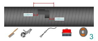
Roughen the surface of the plant coating around the damaged spot with an abrasive pad or sand paper. Remove all contaminations.
