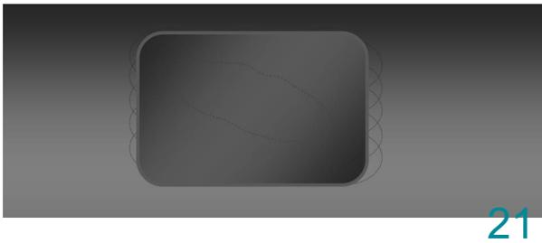
21 The dimpled pattern will disappear when sufficient heat has been applied and some hot melt will protrude from underneath the patch.
