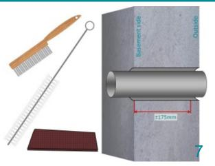
Clean the duct with a brush, cleaning pad or similar equipment. Total length approx. 175mm. Rinse with clean water is allowed as 2100 Aquastop can be applied on a wet surface.
