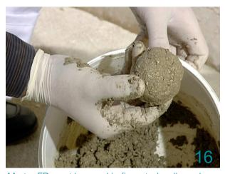
Mortar FR must be used in fire rated walls and floors. Check the malleability of the Mortar FR-WR by moulding the Mortar to a ball shape without it falling apart.
