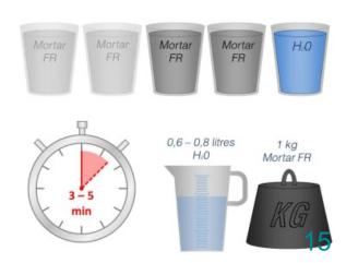
Mixing ratio by weight, mixing time 3-5 minutes: 1 kg Mortar FR and 0,6 – 0,8 litres of water Mixing ratio by volume, mixing time 3-5 minutes: 2 – 4 parts Mortar WR and 1 part of Water.
