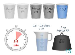
Mixing ratio by weight, mixing time 3-5 minutes: 1 kg Mortar FR and 0,6 - 0,8 litres of water Mixing ratio by volume, mixing time 3-5 minutes: 2 - 4 parts Mortar FR and 1 part of Water.
