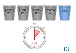
Prepare Mortar WR to a mouldable mass. Mixing ratio by volume, mixing time 1 minute: 4 parts Mortar WR and 1 part of Water.
